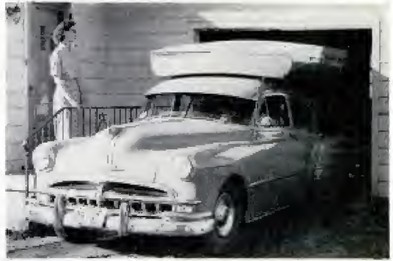
You can drive into your garage with the cabin in place on roof. When you store it, it hangs from the garage rafters above car.
